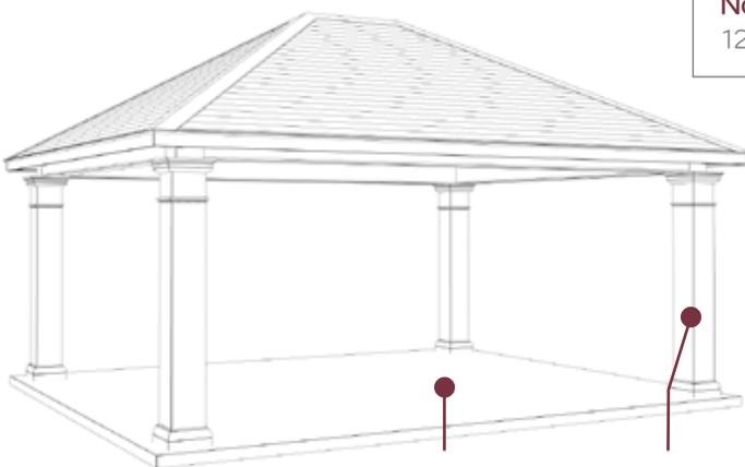
**Note:** Drawing shown with optional 12"x12" fiberglass columns.
