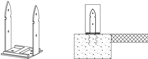
\*Standard bracket includes 3/4" stand-off. In this diagram, the finished patio surface is below the post.
